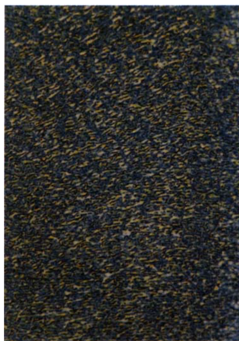
Figure 2. Micrograph under a polarizing optical microscope of the chiral monomer 8a at a magnification factor of \times 320 . Cholesteric texture (38°C) observed by cooling from the isotropic state.
